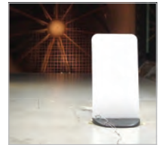
Ecoflex pavement signs tested to Storm Force 10 Beaufort Scale.
